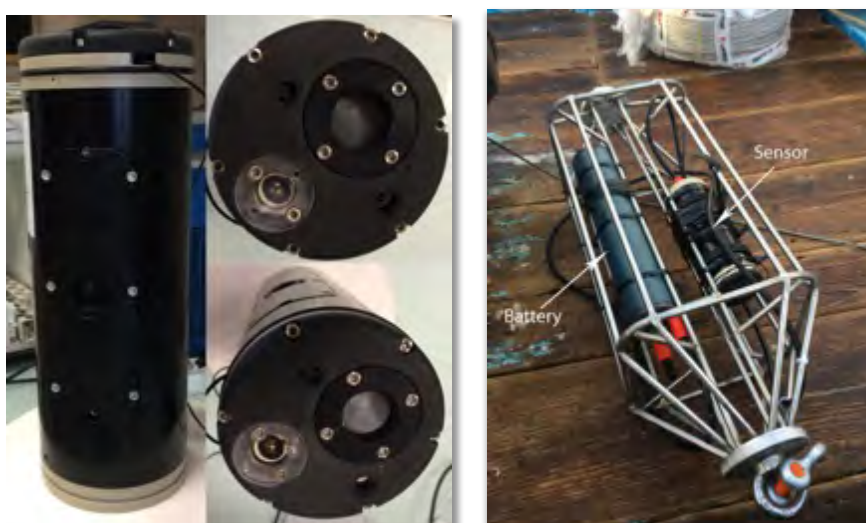
Figure 11. Sensor shown in pressure housing (left). Sensor and power supply mounted on a frame ready for deployment on mooring off the coast of Chile (right)
