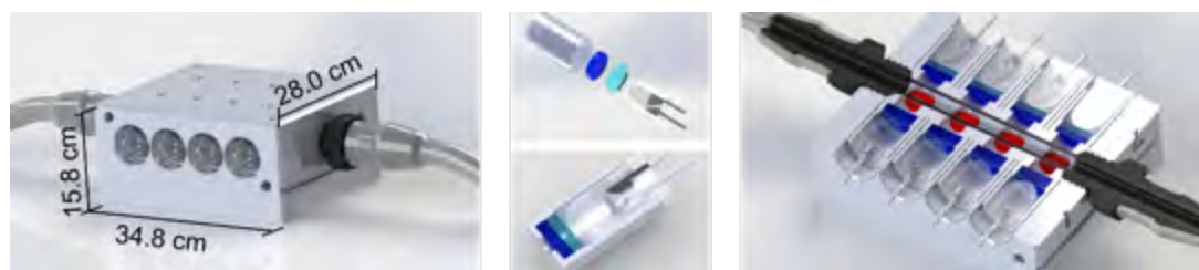
Figure 19 Rendered picture of the algae detection module (left and right) and the modular LED modules used as excitation sources (middle). The picture on the right illustrates the arrangement of optical and electronic components. Photodetectors are aligned with 90° angle to the excitation source and covered with emission filters to minimize cross-talk between excitation and emission channels.
