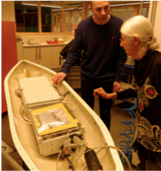
Figure 5. O3 sensor – Cbon2-sv is the upper box in the sailbuoy hull. The vehicle controller is the lower box
